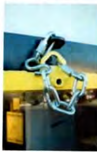
Safety Chain - For safety as well as quick single-person resetting, a safety hook and chain is provided.
