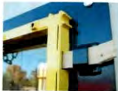
Window Bar Frame Pryable: - Four 1x2 blocks set the frame into place for prying.
